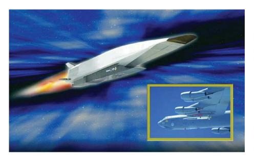
On May 26, 2010, the X-51A Wave Rider made aviation history by completing the longest ever supersonic combustion ramjet-powered flight. The unmanned vehicle flew for almost three and a half minutes in the skies off the southern California coast, reaching an altitude of about 70,000 feet and achieving hypersonic velocity.
